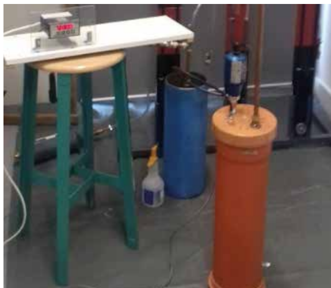
Figure 12. Open vented containment set up.
