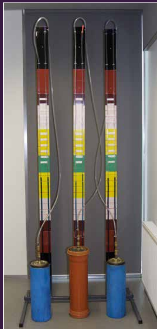
Fig. 3 Burke Oxygen depletion experiment set up (BODE)
