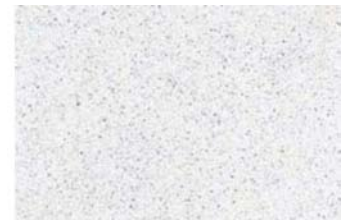
White acid washed precast concrete
