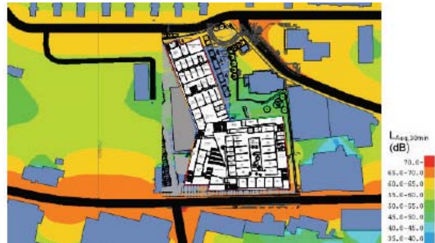
Noise analysis: predicted levels +14.0m above ground level
