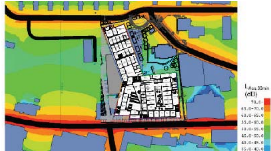
Noise analysis: predicted levels +1.5m above ground level
